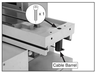
Figure 17. Cable barrel attached.
